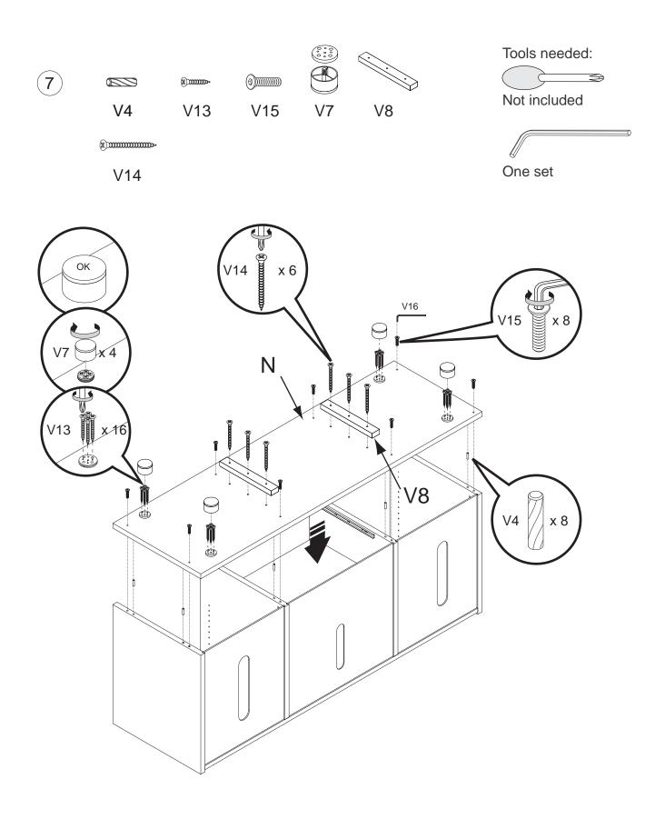
Attach bottom board (N) to the TV cabinet body with screws (V15)and wooden dowel(V4). Attach feet (V7) to the bottom board (N) with screws (V13). Attach wood bar (V8) to the bottom board (N) with screws (V14). After the feet are assembled, turn the whole unit over and make it stand upright.
